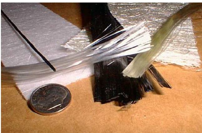
Examples of various reinforcement materials used in polymeric composites
