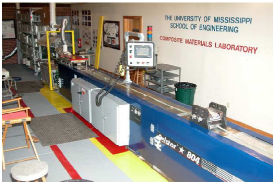
Pultrusion machine in the composite materials manufacturing lab
