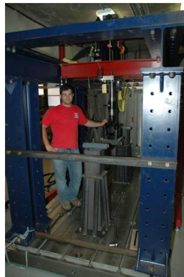
Student standing in the biaxial free form mechanical test frame
